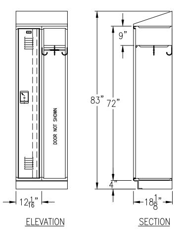
PLEASE BE ADVISED: Lockers Are Square And Measured Based On Square Walls. If Walls Are Not Square, Adjustments To Bases
