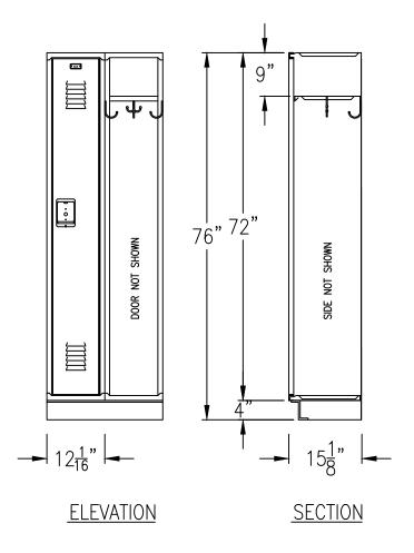
PLEASE BE ADVISED: Lockers Are Square And Measured Based On Square Walls. If Walls Are Not Square, Adjustments To Bases Will Need To Be Made At The Expense Of The Customer To Make Allowances For The Locker Sizes As Specified In The Shop Drawings.
