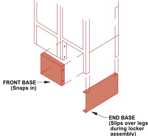
Front and End bases are designed to fit between standard Lockers Manufacturing 6" legs. They present a clean flush appearance and prevent the accumulation of dust and dirt under the lockers. (Not for use on All Welded lockers). Front base snaps in. End base slips over legs during locker assembly.
